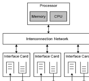
Fig 1. Router components.
