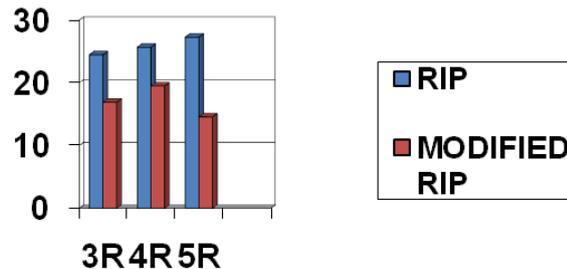
Fig 10 Graph of the comparison of packet loss with 3, 4 & 5 routers
