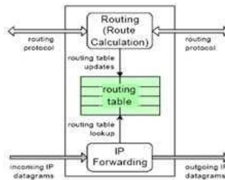
Fig 2. Functions of a router.
