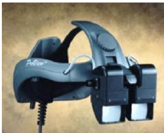
Fig. 2: Optical See-Through HMD
