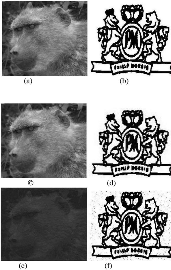
Figure 5: MATLAB and Xilinx Embedding De-embedding Outputs, (a) Cover Image, (b) Secrete Image, (c) Embedded image from MATLAB, (d) extracted Image from MATLAB, (e) Embedded image from Xilinx, (d) extracted Image from Xilinx.
