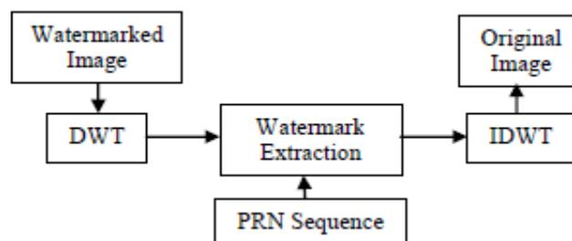
Fig 3: Block diagram of watermark extraction.
