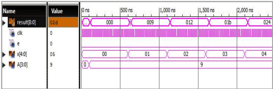
Fig.4: Simulation result of APC based LUT multiplier for L=5
