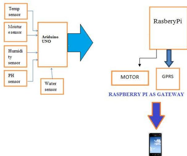
Figure 1. Proposed Automation of Irrigation System.
