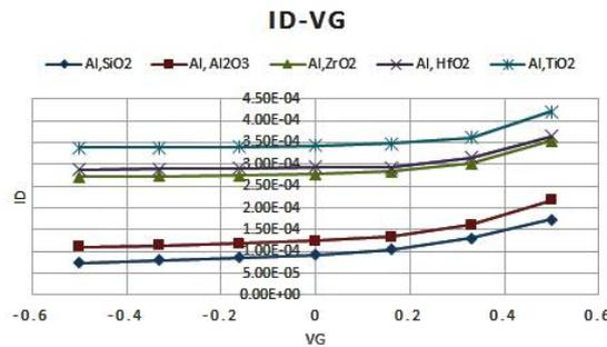
Figure 4:  $I_D$ - $V_G$  of curved DG MOSFET (with Al-Gate,  $V_{GB}=0.5V$ ,  $l=45nm$ ,  $t=2nm$ ,  $N_D=2*10^{20}cm^{-3}$ ,  $L_{SD}=50nm$ ,  $t_{ch}=30nm$ , at  $V_D=1V$ )
