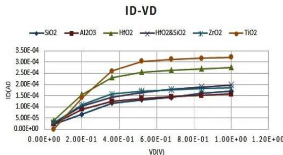
Figure 5:  $I_D$ - $V_D$  of rectangular DG MOSFET (with Al-Gate,  $V_{GB}=0.5V$ ,  $l=45nm$ ,  $t=2nm$ ,  $N_D=2*10^{20}cm^{-3}$ ,  $L_{SD}=50nm$ ,  $t_{ch}=30nm$ , at  $V_D=1V$ )
