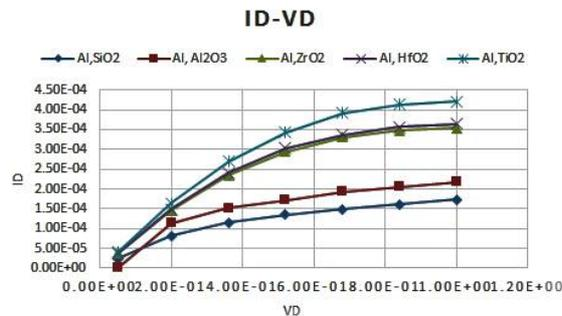
Figure 6:  $I_D$ - $V_D$  of curved DG MOSFET (with Al-Gate,  $V_{GB}=0.5V$ ,  $l=45nm$ ,  $t=2nm$ ,  $N_D=2*10^{20}cm^{-3}$ ,  $L_{SD}=50nm$ ,  $t_{ch}=30nm$ , at  $V_D=1V$ )
