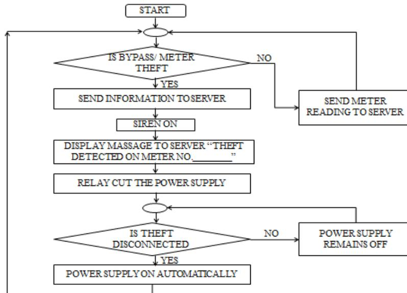
Above flowchart is used to detect power theft at pole as well as at consumer meter in following way;
