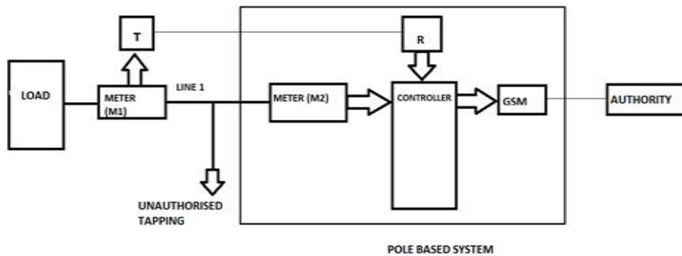
Fig (1). Block diagram of power theft detection.
