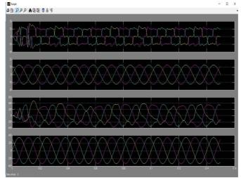
Fig: 6 iUPQC transitory response during the connection of a threephase diode rectifier: (a) load currents, (b) grid currents, (c) load voltages and (d) grid voltages.
