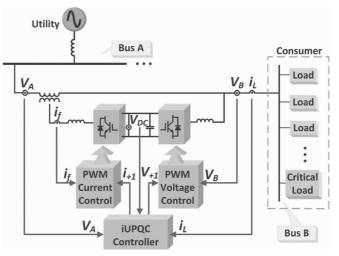
Fig. 2. Modified iUPQC configuration
