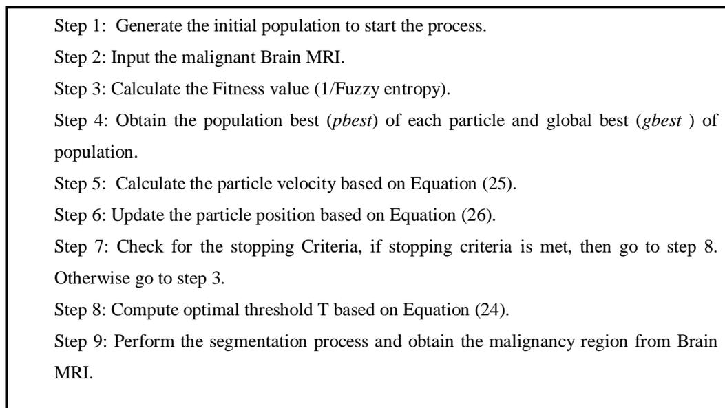
Figure 3. Algorithm for MPSO based fuzzy entropy MR Brain malignancy segmentation
