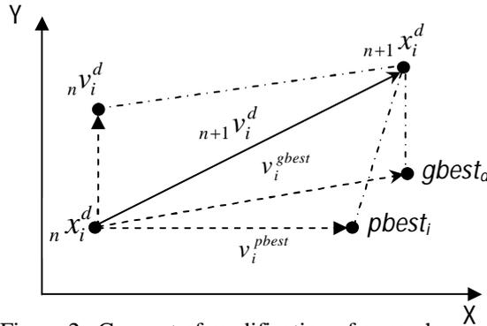
Figure 2. Concept of modification of a search position by PSO
