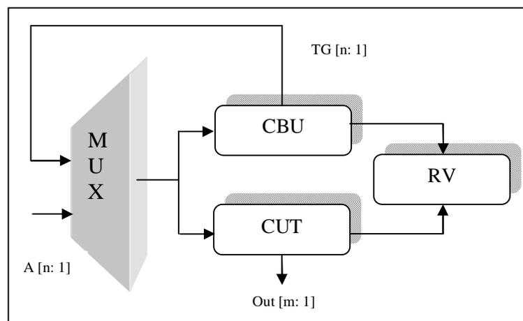
Fig.2 Input vector monitoring concurrent BIST architecture
