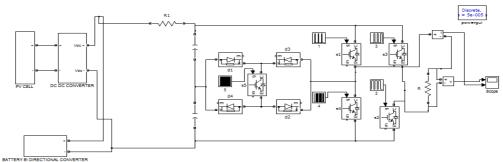
Fig.12 Simulink model of five level inverter
