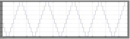
Fig 17 Simulation wave form nine level inverter output
