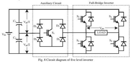
Here an auxiliary circuit consists of one switch and four diodes are used along with a full bridge configuration. The principle of operation of the proposed inverter is to generate five levels of output voltage, V/2, V, 0; -V/2 and -V. Using proper switching sequence in this modified circuit, five levels in output voltage is generated [10]. Table 1 shows the switching sequence used for generating five levels in the output voltage.
