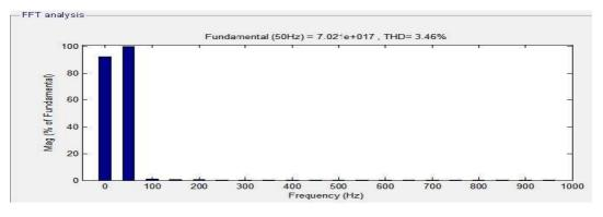
Fig.7. Total harmonic distortion of inverter current
