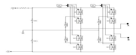
Fig.2. NPC Three level inverter model
