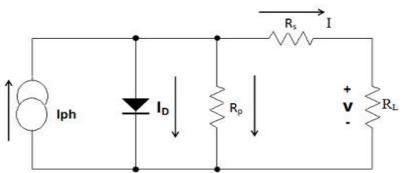
Fig.3. PV single diode model
