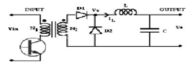
Fig2. Forward converter
