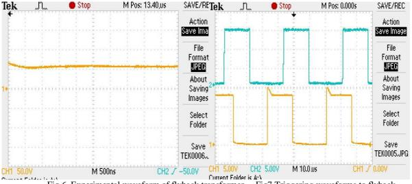
Fig 6 Experimental waveform of flyback transformer Fig7 Triggering waveforms to flyback
