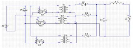
Fig 3.Three celled interleaved flyback topology
