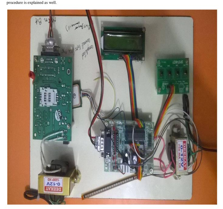
This is a whole setup of the block diagram. When the input sensor is bent, the bending effect will be increased over the set value it activates the microcontroller, which is connected to the GPS and GSM. The GSM gets the location from the GPS and sends an emergency notification.
