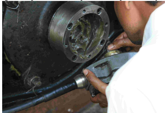
Fig6: Installation of wheel sensors
