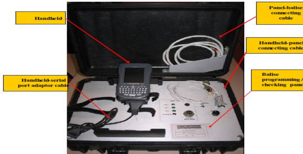
Fig5: Components of Balise Programming Verification Tool
