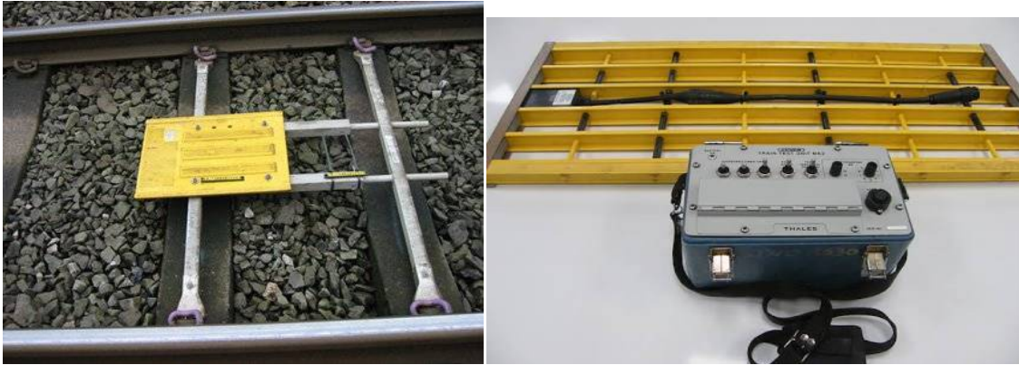
Fig2: Eurobalise installed on track and close view
