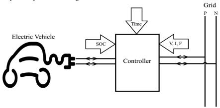
It consists of mainly a self-controlled controller and other electrical & electronic circuits to perform charging and discharging operation. Self-controlling of the controller is purely based on certain parameters like Grid Voltage, Current, Frequency, State Of Charge of Battery and time. Since the aim of the paper is to facilitate DSM, time is set as the main base of the controller operation.
