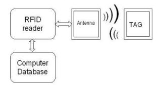
Fig. 3: Block diagram of working of RFID
