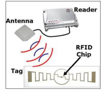
Fig.1: Basic RFID
