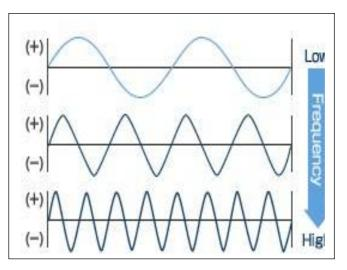
Fig. 2: Time domain representation of different frequency levels
