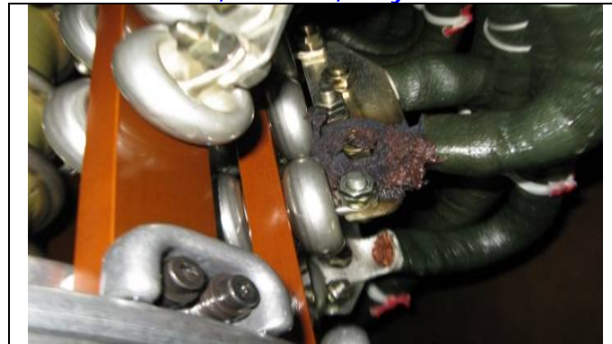
Figure 7. The point of Incipient fault for case B
