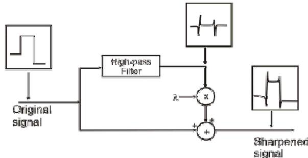
Figure 2:Sharpening Filter
