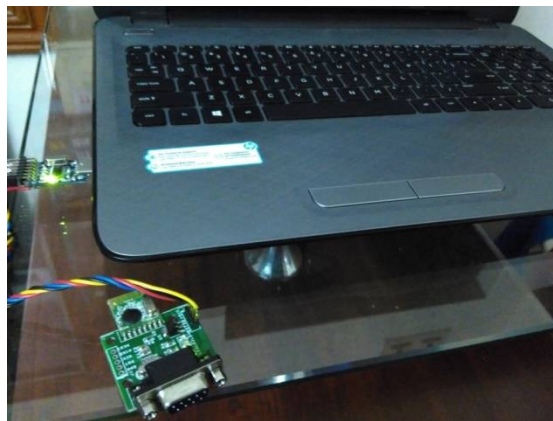
Fig. 6 Zigbee receiver interface to PC using USB-UART converter
