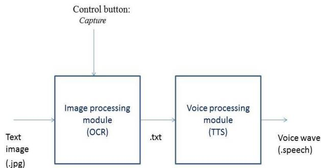
Fig.3 Block Diagram of Text-To-Speech Device
