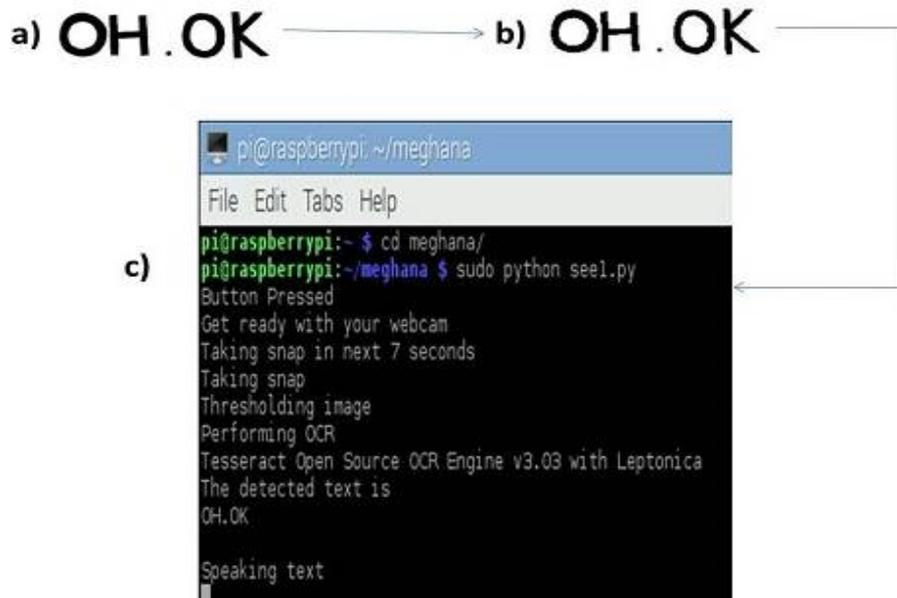
Fig.7 a) captured image with white background b) threshold image c) output
