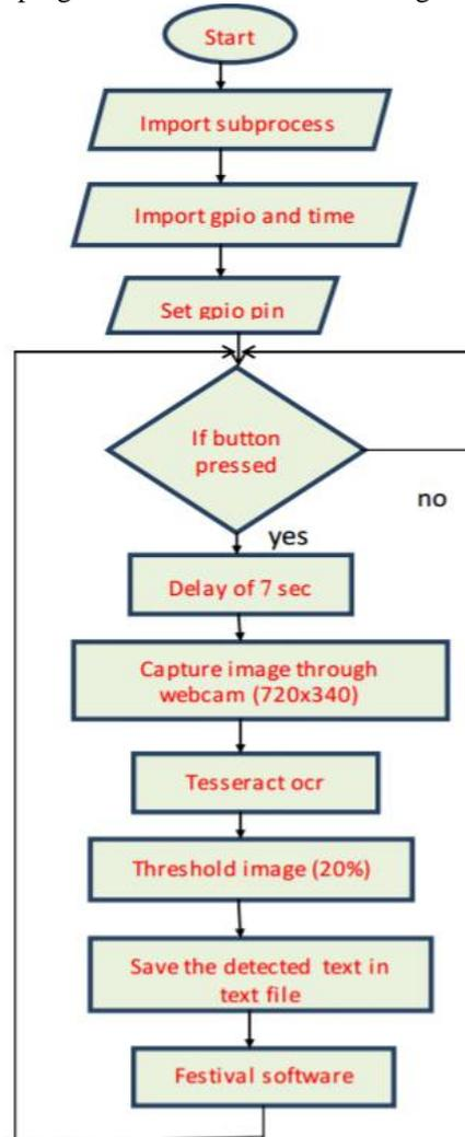
Fig.5 Flow chart of text-to-speech device program
