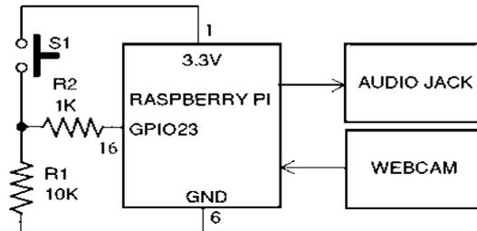
Fig.2 Circuit connection to Raspi board
