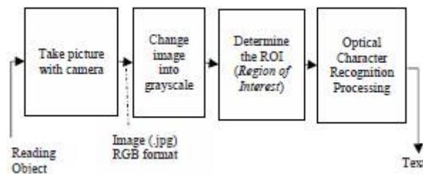
Fig.4 Software Design of Image Processing Module
