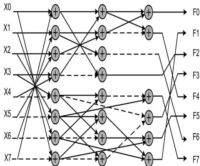
Fig.1 SIGNAL FLOW GRAPH (SFG) OF (C8)
