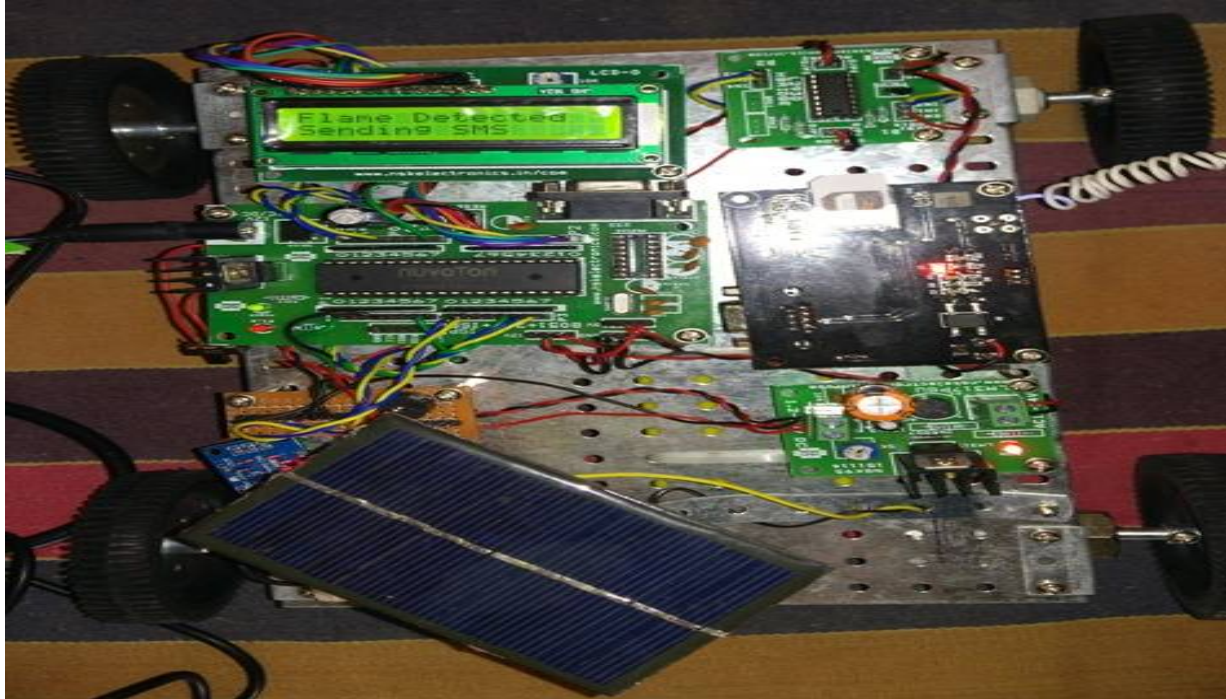
Figure 3 . shows the Automatic Fire Detection using GSM and image Proceesing ,it consists of gsm ,lcd,solar panel, 5v battery, h-bridge, 2v dc motors,water pump and storage tank.
