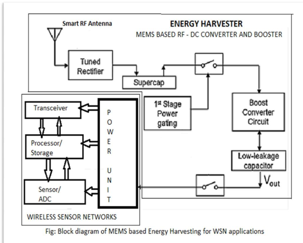
The output thus obtained can be directly or converted in to require form may be used to power ultra-low power electronic devices and sensors. The signal can also be transmitted in to the wireless sensors, processed for low power programmable applications etc. With the advancement in wireless communication technologies, inexpensive and ultra-low power wireless sensors can be developed. Hence the harvested energy can be utilized for wireless sensing applications.
