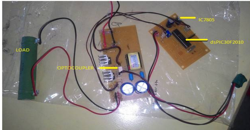
Fig 8: Hardware implementation of flyboost converter with PI controller
