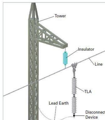
Figure 6 Transmission Line Arrester installation in tower: Case (c) parallel to the insulator.
