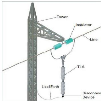
Figure 4 Transmission Line Arrester installation in tower: Case (b) beside the insulator.
