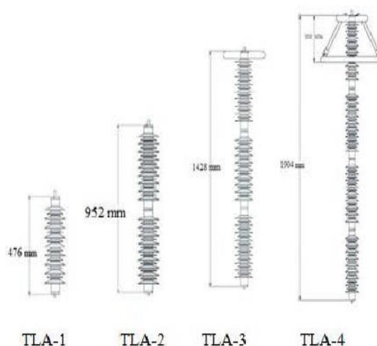
Figure 3 Dimension of Transmission Line Arresters [6].
