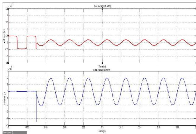
Figure 9 Voltage and Current waveform at load side (8 MW).
