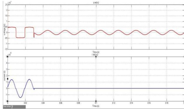
Figure 7 Voltage and Current waveform at MOV 1.
