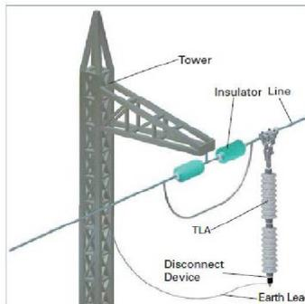
Figure 5 Transmission Line Arrester installation in tower: Case (a) across the insulator.
