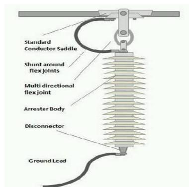
Figure 2 Typical suspension lightning arrester [5]
