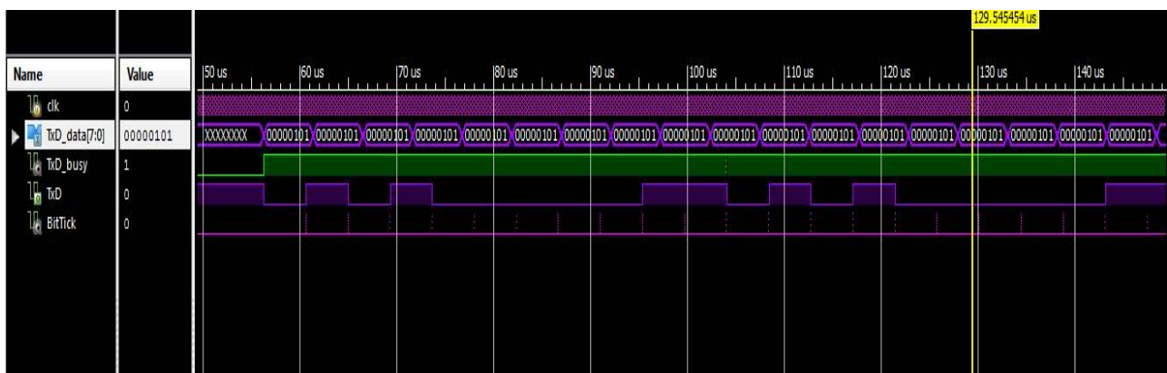
Fig. 5 Simulation result of UART transmitter
