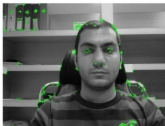
Figure 9: Extracting the main image key points through FAST
