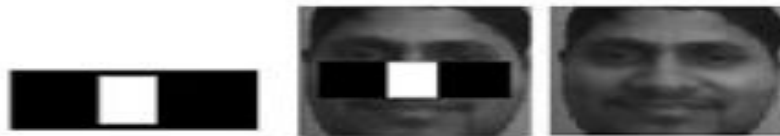
Fig-4.2.1.a: Haar Feature that looks similar to the bridge of the nose is applied onto the face
