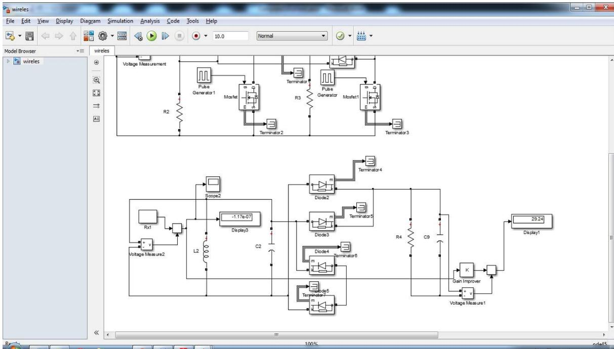
Figure.9. Receiver End - Detailed View
