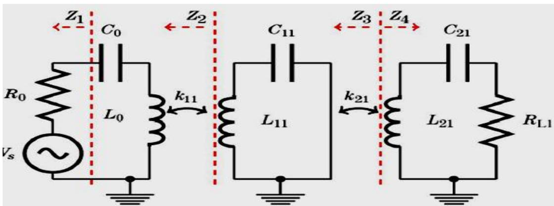
Figure.4. Equivalent circuit for wireless power transfer with repeater
