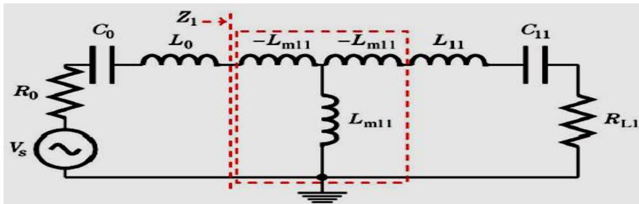
Figure.2. Impedance Inverter as Coupling Strength Representation
