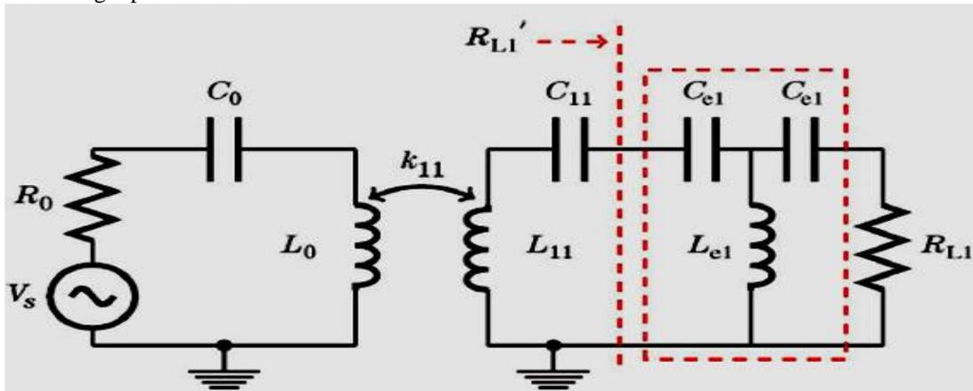
Figure.3. Impedance Inverter for Impedance Transformation
