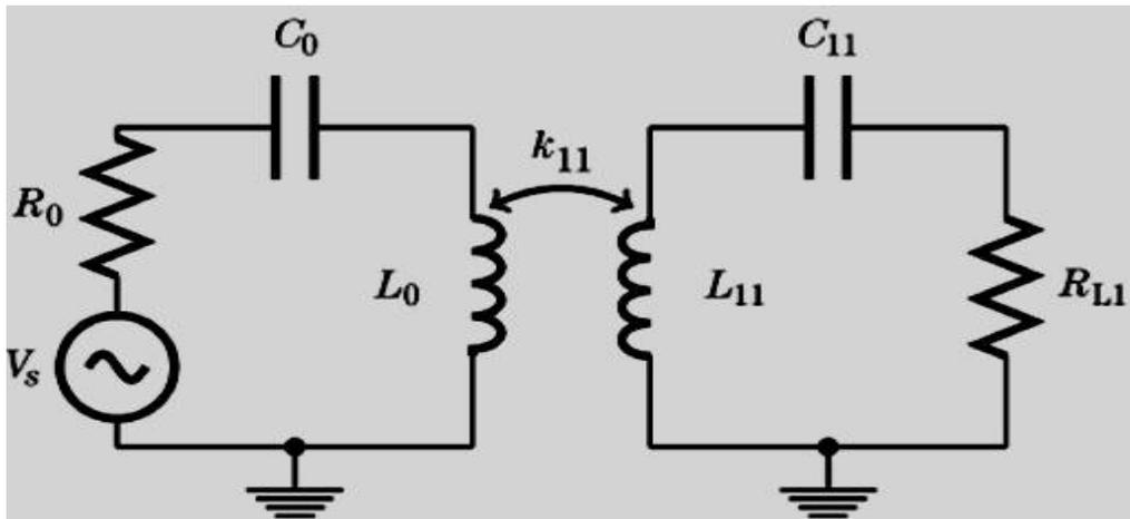
Figure.1. One End Transmitter and Receiver Wireless Power Transfer
