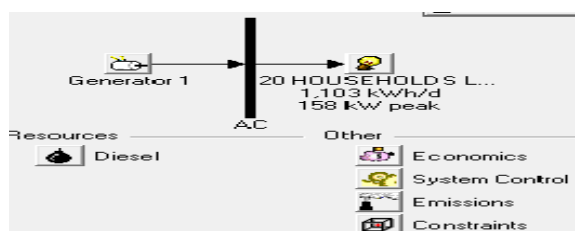
Fig.11 Diesel connected power System
