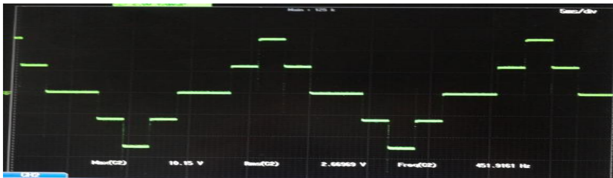
Fig.11.Output voltage across R load
