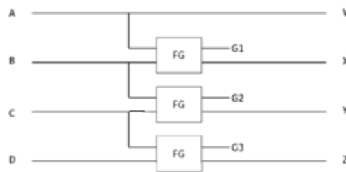
Figure 11. Circuit diagram of Reversible Binary to Gray code converter.
