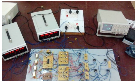
Figure 11: Hardware Setup for MSPWM based Seven Level Inverter
