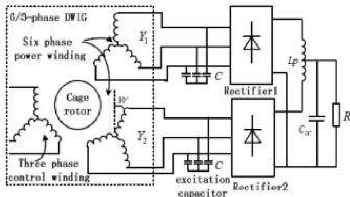
In the DWIG, two sets of stator windings are present, and an SEC is connected to the control winding, which results in increased complexity of the voltage buildup process when compared with a traditional IG. Considering that no-speed sensor exists in this system, the entire voltage buildup process is divided into three steps, namely, frequency search, generation in an open loop, and generation in a closed loop.
