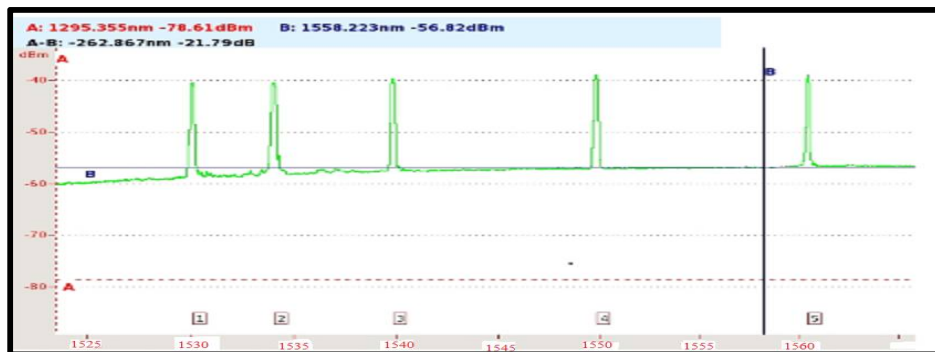
Fig. 6 Output spectrum of five different FBG sensors.
