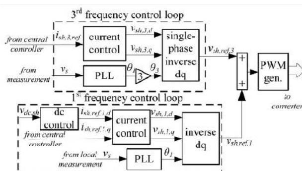
Fig. 8. Block diagram of the shunt converter control.
