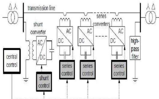
Fig. 6: DPFC control block diagram.
