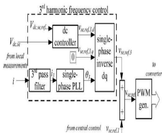
Fig. 7: Block diagram of the series converter control.
