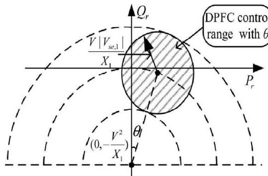
Fig. 5: DPFC active and reactive power control range with the transmission angle  $\theta$ .
