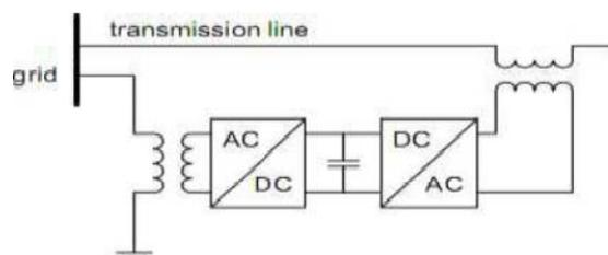
Fig.1: Simplified representation of a UPFC
