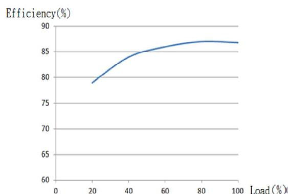
Figure 3. A plot of the LED driver efficiency versus load.
