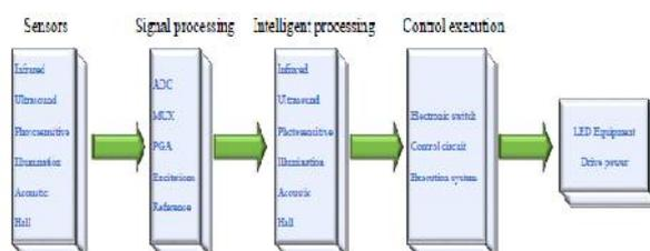
Figure 2. Operation sequences of a smart LED lighting system.
