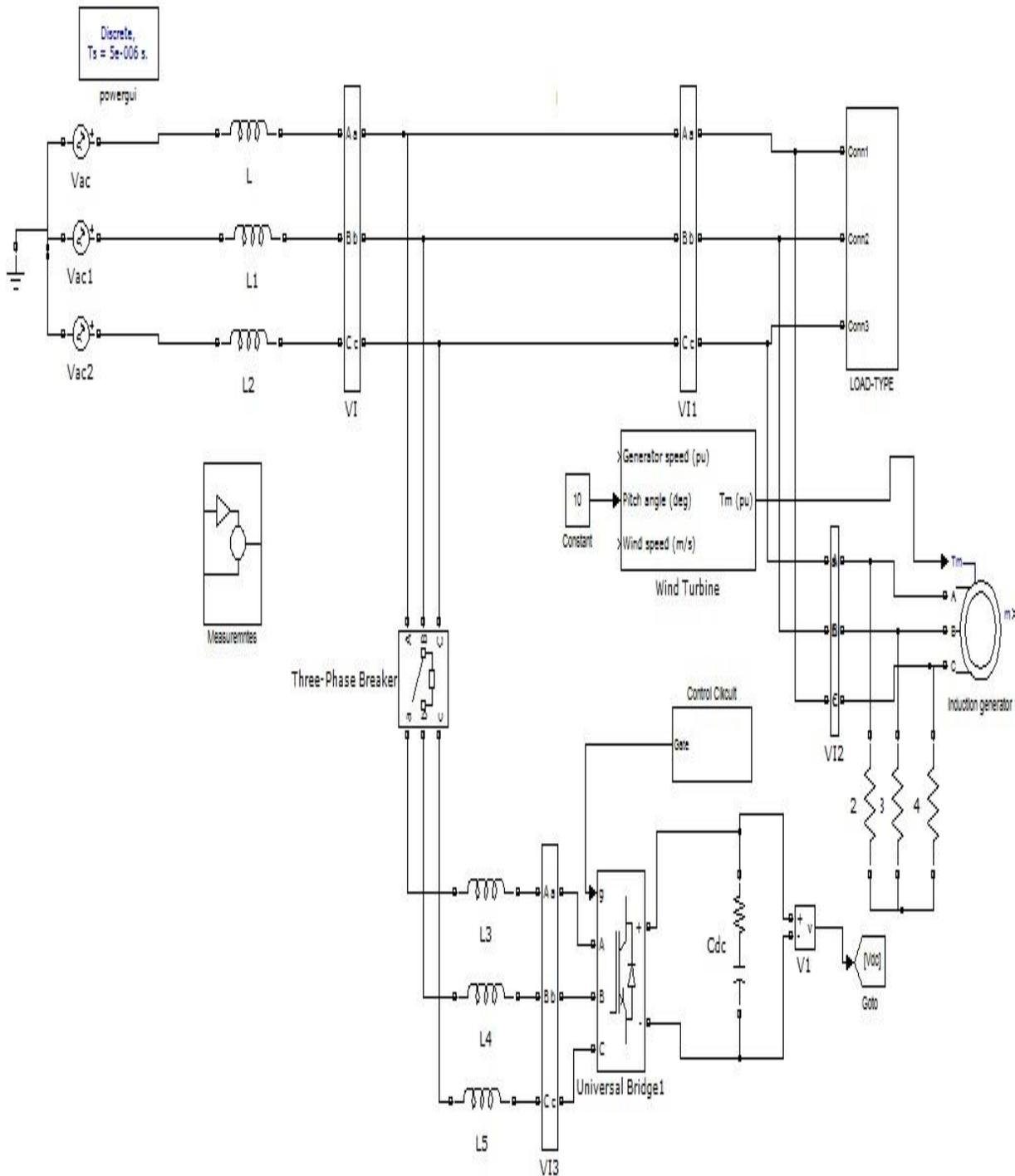
Fig.5. Matlab /Simulink of Proposed STATCOM-Power Circuit
