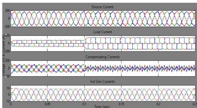
Fig. 18 shows the Simulation results of Variable Load, source current, load current and compensator current and induction generator currents
