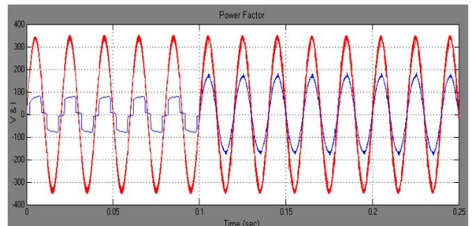
Fig.11 Simulation Results Power Factor For Balanced Non- Linear Load
