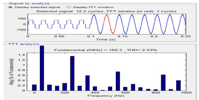
Fig. 13 FFT Analysis of Phase-A Source Current for Balanced Non-Linear Load
