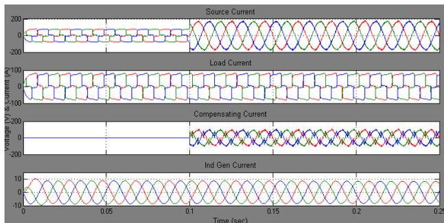
Fig.10 Simulation results for Balanced Non Linear Load (a) Source current. (b) Load current. (c) Compensator Current. (d) Wind Generator (Induction Generator) Current.
