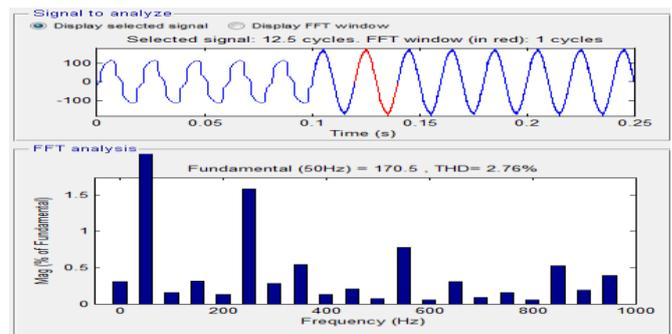
Fig. 17 FFT Analysis of Phase-A Source Current for Un-Balanced Non-Linear Load
