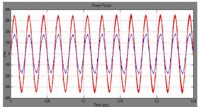
Fig. 19 Simulation Results Power Factor For Variable Load Condition Fig. 19 shows the power factor it is clear from the figure after compensation power factor is unit
