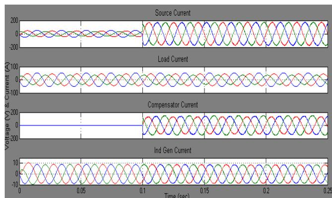
Fig. 8 Simulation results of Linear Unbalanced Load (a) Source Current (b) Load Current (c) Compensator Current (d) Wind Generator (Induction Generator) Current.
