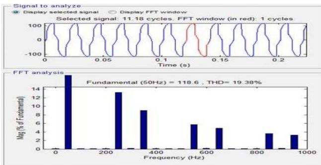
Fig.16 FFT Analysis of Phase-A Source Current for Un-Balanced Non-Linear Load
