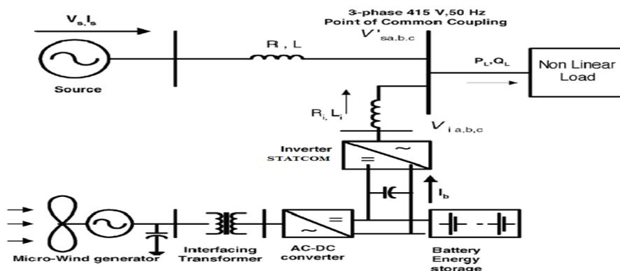
Fig.1 Scheme of wind generator with battery storage [6].
