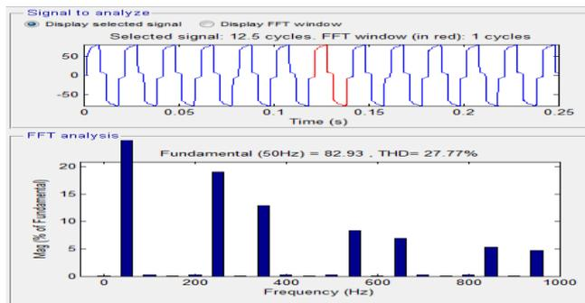
Fig. 12 FFT Analysis of Phase-A Source Current for Balanced Non-Linear Load
