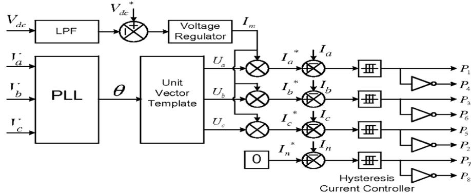
Fig. 3. Block diagram representation of grid-interfacing inverter control.
