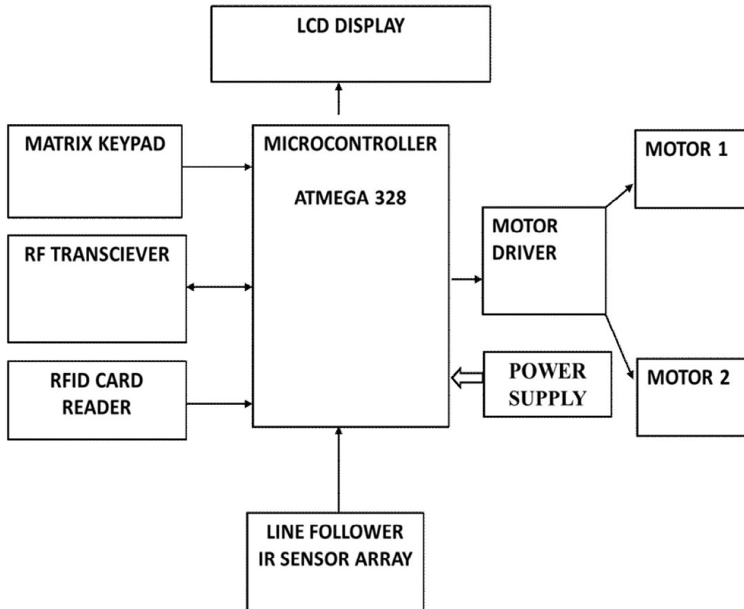
Fig. 2. ROBOT END BLOCK DIAGRAM
