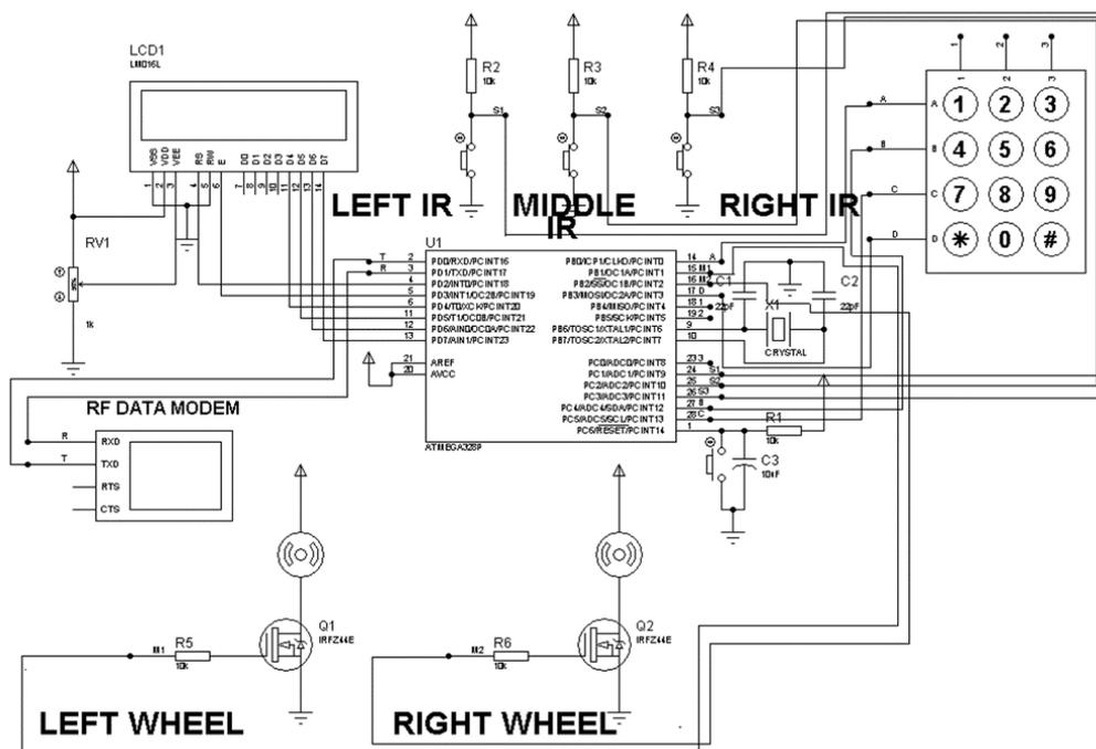
Fig. 4. Circuit diagram
