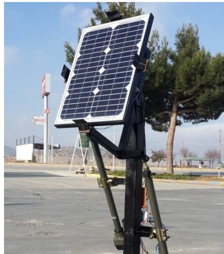
Fig. 5 View of the two axis tracking system
