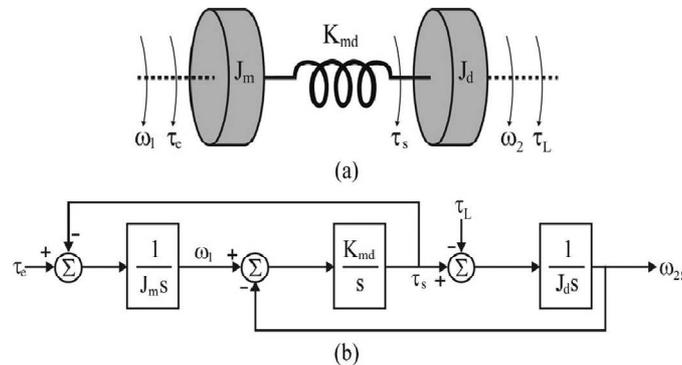
Fig.1. Mechanical schematic of a two-mass system.
