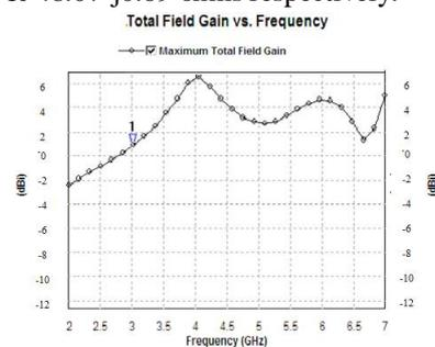
Figure 21: Variations in Gain with frequency for modified microstrip patch Antenna loaded with two pair of slits
