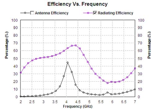
Figure 23: Variations in antenna efficiency & radiating efficiency with frequency for modified microstrip patch Antenna loaded with two pair of slits
