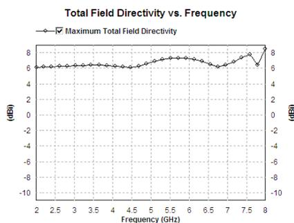
Figure 15: Variations in field directivity with frequency for modified microstrip patch Antenna loaded with one pair of slits
