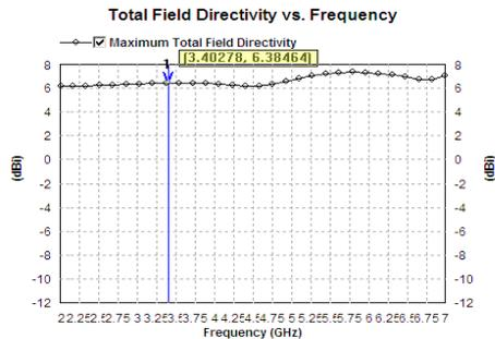
Figure 6: Variations in Field directivity with frequency for proposed antenna
