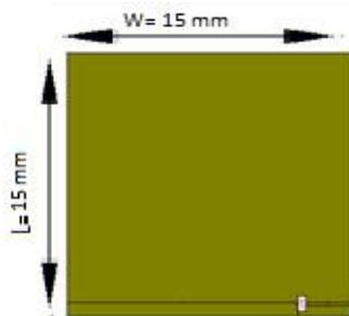
Figure 1: Geometry of proposed microstrip patch antenna
