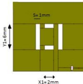
Figure 10: Geometry of modified microstrip patch Antenna loaded with one pair of slits
