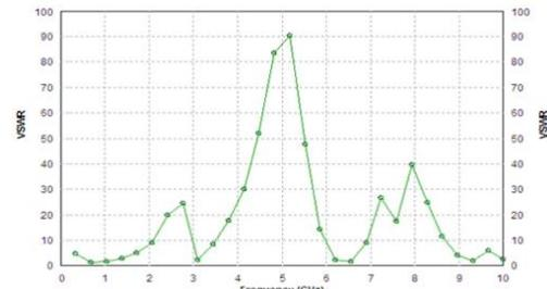
Figure 26: Variations in VSWR with frequency for modified microstrip patch Antenna loaded with three pair of slits
