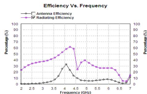
Figure 30: Variations in antenna efficiency & radiating efficiency with frequency for modified microstrip patch Antenna loaded with three pair of slits
