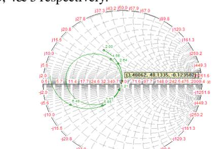
Figure 5: Variations in input impedance with frequency for proposed antenna
