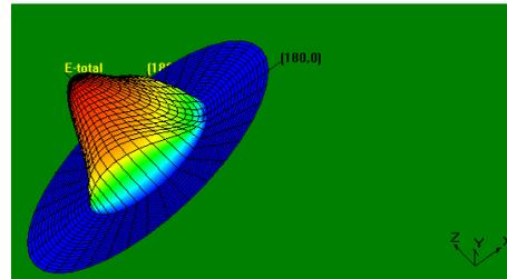
Figure 9: 3D representation for proposed antenna
