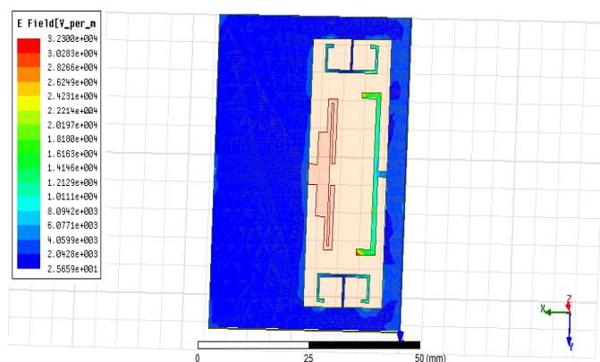
Figure 3.4 E-Field distribution in the frequency range 2.56-3.23 GHz
