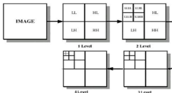
Fig 3: four level wavelet decomposition
