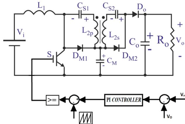
Fig. 2. Circuit Diagram - A Closed loop model of modified SEPIC converter with magnetic coupling and output diode voltage clamping.
