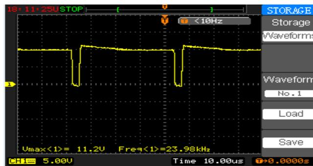
Fig. 16. Output waveform of the drive circuit
