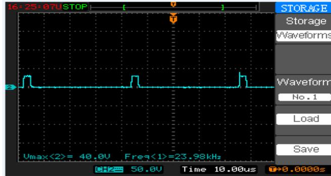
Fig. 18. Switch voltage waveform of the proposed converter
