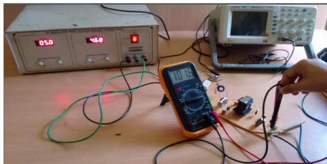
Fig. 17. Experimental set-up:A closed loop model of SEPIC converter with magnetic coupling and output diode voltage clamping
