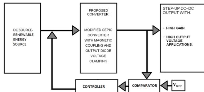
Fig. 1. Block Diagram – A Closed loop model of modified SEPIC converter with magnetic coupling and output diode voltage clamping
