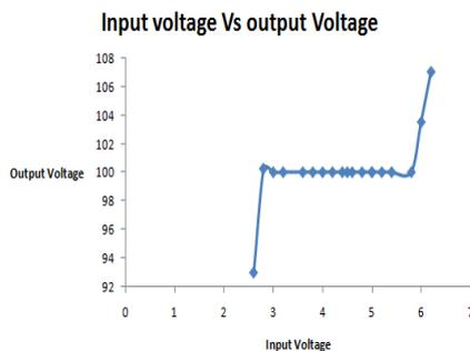
Fig. 20. Closed loop Simulation at constant load
