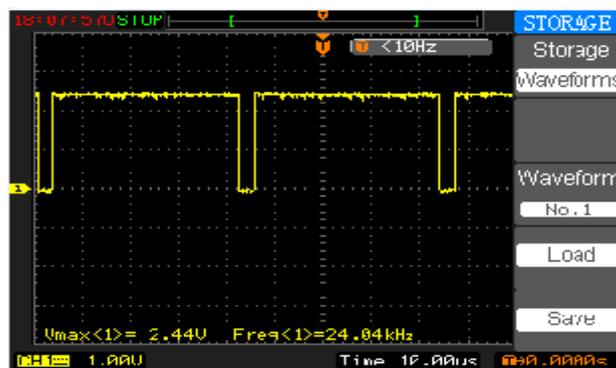
Fig. 14. Output waveform from the control circuit
