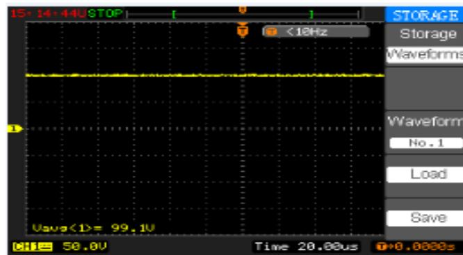
Fig. 19. Output voltage waveform of the proposed converter
