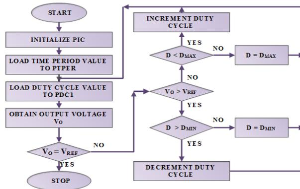
Fig. 12. Closed Loop Program Flow Chart
