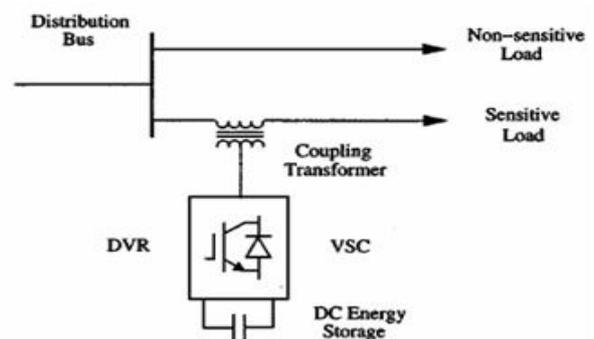
Fig 8. Schematic representation of the DVR
