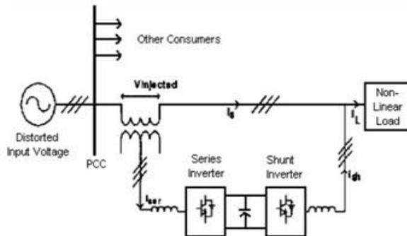
Fig 9 Basic Block Diagram of UPQC
