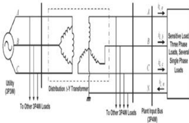
Fig. 11 3P4W distribution system: neutral provided from Δ-Y transformer
