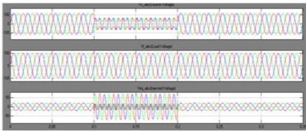
Fig 19. Simulation results using conventional topology. Terminal voltages with sag, DVR-injected voltages, and load voltages after compensation
