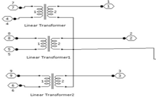
Fig. 16. Simulink diagram of three-phase series Transformer
