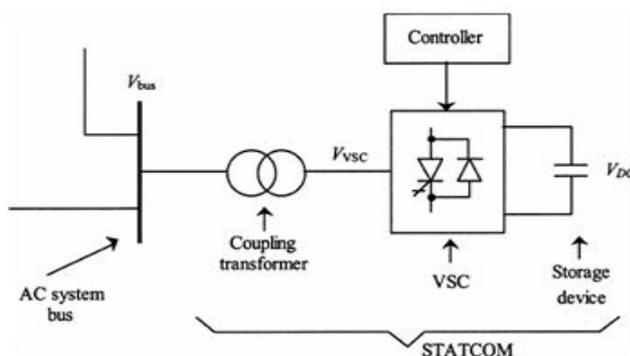
Fig 7. Schematic representation of the DSTATCOM
