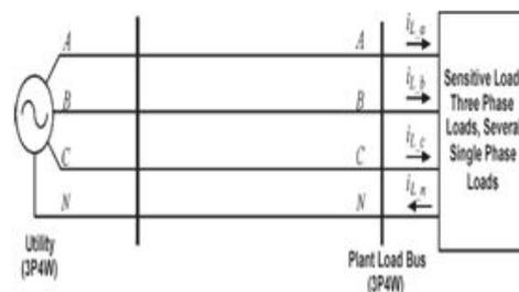
Fig. 10 3P4W distribution system: neutral provided from generation station
