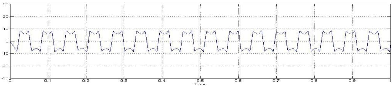
Fig. 6 Back EMF waveform.
