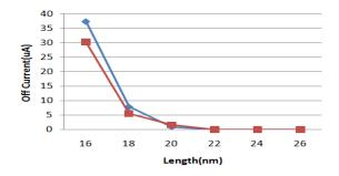
Fig. 3 Off current comparison of DG MOSFET(blue) and TG FinFET(red) as a function of gate length
