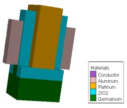
Fig. 4 DG MOSFET with high-k dielectric
