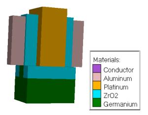
Fig. 5 Trigate FinFET with high-k
