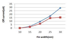
Fig. 1 Off current comparison of DG MOSFET(blue) and TG FinFET(red) as a function of fin width
