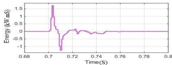
Fig.10. Transient energy during rectifier fault
