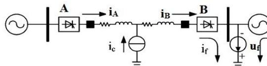
Fig. 4. Effect of shunt capacitance
