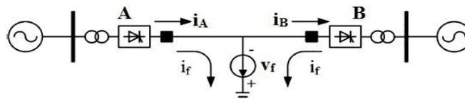
Fig.5. Internal fault
