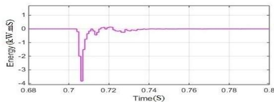
Fig.12. Transient energy during DC line fault
