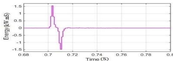
Fig.11. Transient energy during inverter fault
