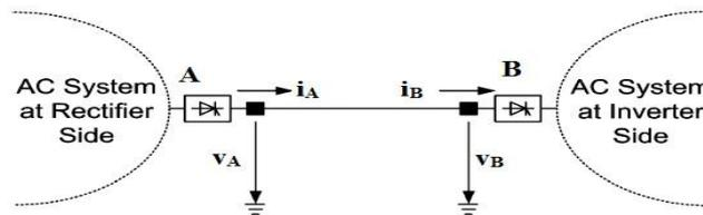
Fig.1. Typical structural diagram of HVDC system
